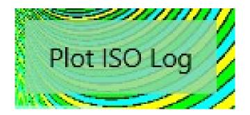
Pressing the 'Plot ISO Log' uses the same ISO algorithm but replaces each scalar field value with the logarithm value. Plot(Log(value)) instead of Plot(value).
